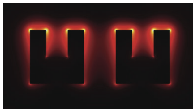
Figure 14 (online color at: www.lpr-journal.org ) Absolute value of the time-harmonic electric field in a plane through the centre of the SRR dimer with d = 120 nm. Note the strongly localised fields near the sharp corners.
